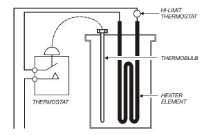
Fig. 3 Heat Control Diagram
